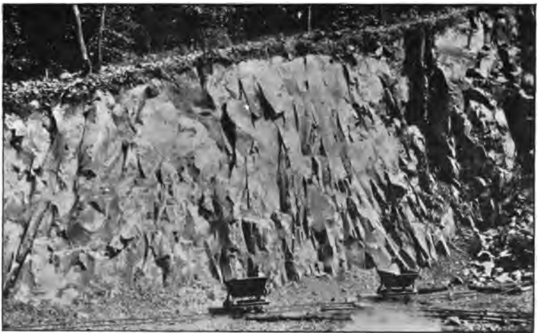
Fig. 2. Irregular jointing in basalt of Second Mountain. Quarry, 1 mile south of West Summit.
